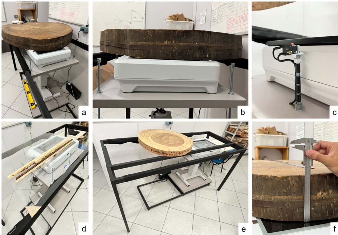
Figure 2. Final equipment scanning table system: (a) scanner table system with sample >85 cm in diameter, (b) side view of the sample above the scanner, (c) protection tower with limit switch, (d) glass for increment cores > 42 cm (accessory 1), (e) transversal support bar for 60 to 80 cm discs (accessory 2), and (f) measurement of the distance between the wooden sample and the scanner glass.
